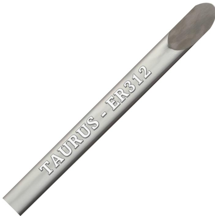
TAURUS TIG 312 rod has good oxidation resistance at high temperatures due to its high content of Chromium. The alloy is widely used for joining dissimilar steels, especially if one of the components is fully austenitic, and for steels that are difficult to weld, like for example machine components, tools and austenitic manganese steels.
