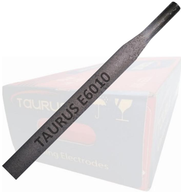
TAURUS PRO 6010 is a medium coated, DC, cellulosic electrode for welding vertical down in pipeline and storage tank construction. Recommended for root-filler layers in pipeline applications. An extremely fast deposition rate can be obtained applying a touch or short-arc technique. The electrode provides a very steady arc over a wide range of current values.
