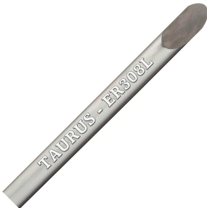
TAURUS TIG 308L rod is used for welding 18/8 stainless steels including 301, 302, 303, nitrogen-bearing 304LN and similar. Service temperatures are typically -100°C to approximately 400°C.
