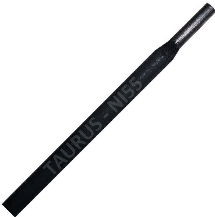
TAURUS PRO Ni 55 is an all positional electrode depositing a 55% Ni/45 % Fe weld metal designed specially for strength welding of grey cast iron and malleable cast iron with steel. Also designed to operate at low current which minimises heat input and thus facilitates the cold welding of cast iron. Weld induced stresses can be reduced by hammer peening. Stable arc with clean bead appearance. The weld metal is fully machinable.
