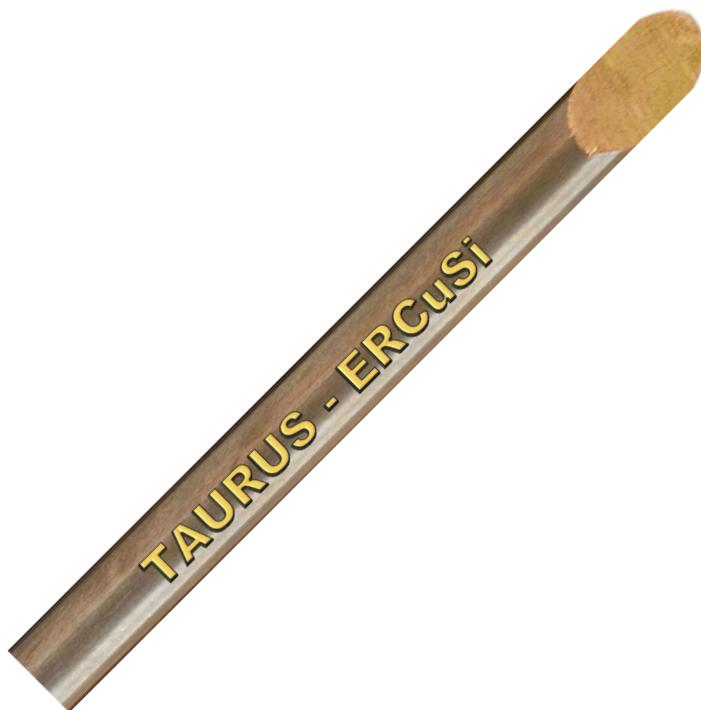
TAURUS TIG SILICON BRONZE is pure copper filler rod deoxidised with 3% silicon for welding a wider range of copper alloys including overlaying of steels and cast irons. TAURUS TIG SILICON BRONZE should be shielded with pure argon but pure helium provides deeper penetration, higher travel speeds and allows reduced preheating.
