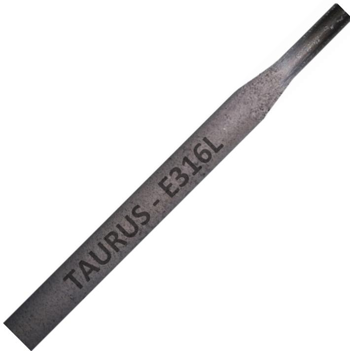
TAURUS PRO 316L is a rutile, high-alloy, extra-low carbon austenitic electrode for welding corrosion resistant CrNiMo steels resistant to atmospheric corrosion. Resistant to grain disintegration at operating temperatures up to 350°C. Very smooth weld with clean weld edge, low spatter loss and easy slag removal. Suitable for welding AISI/ASTM 316, 316L, 316LN, 316H and 316Ti.
