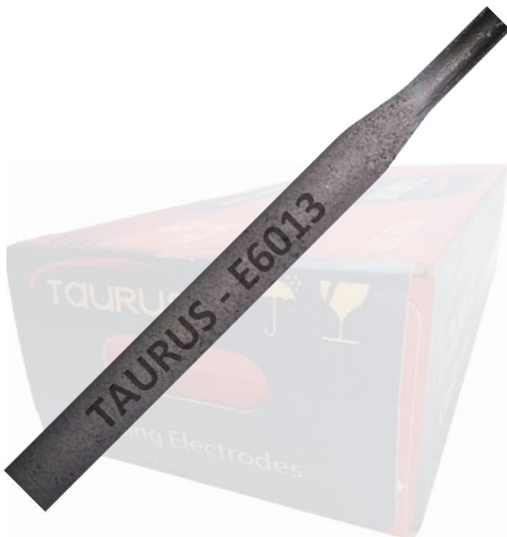
TAURUS PRO E6013 is a rutile-cellulosic type stick electrode designed for a wide range of general fabrication applications for workshop and site conditions. Excellent operability in all positions including vertical down. Particularly suited where poor fit-up conditions prevail. Easy slag removal and low spatter loss. Weld bead appearance is smooth with a fine ripple formation.
