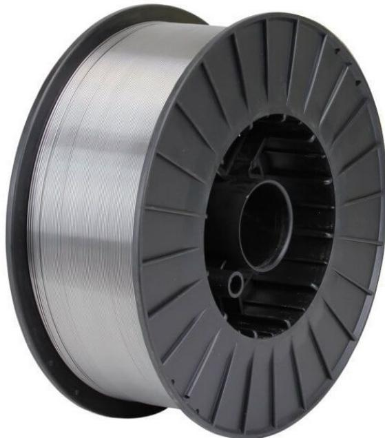
Taurus aluminium-bronze MIG wire is an intermediate-strength alloy with improved resistance to wear and brazing. It is used for aluminium-bronze plate fabrications and for dissimilar metals such as cast iron, carbon steels, copper as well as copper-nickel materials.
