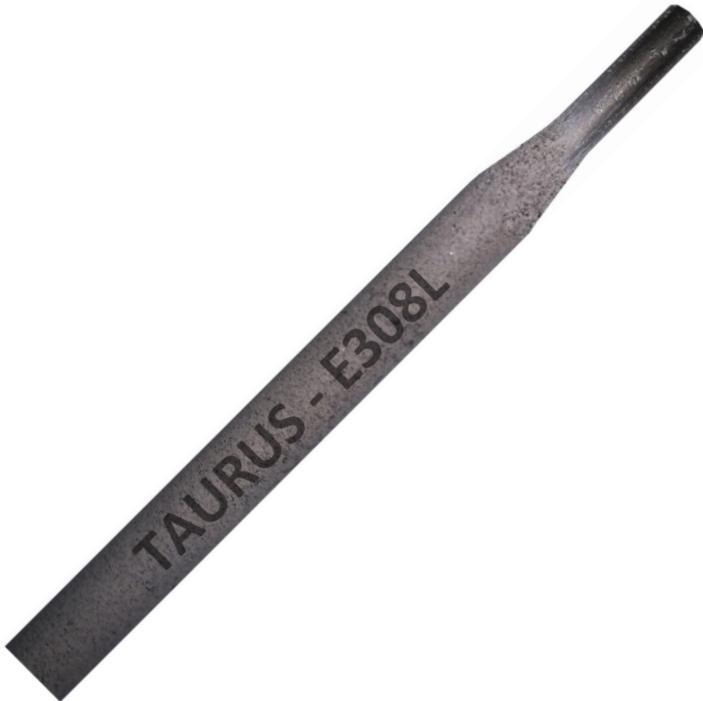
TAURUS PRO 308L is a general purpose, extra-low carbon, austenitic electrode with rutile coating for welding corrosion-resistant CRNi steels. Resistant to atmospheric grain disintegration at operating temperatures up to 350°C. Very smooth weld with clean weld edge. Low spatter loss and easy slag removal. Suitable for welding AISI 302, 304, 340L and 304LN.
