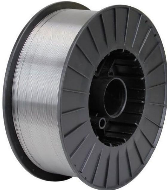
TAURUS MIG 312 wire has good oxidation resistance at high temperatures due to its high content of Chromium. The alloy is widely used for joining dissimilar steels, especially if one of the components is fully austenitic, and for steels that are difficult to weld, like for example machine components, tools and austenitic manganese steels.
