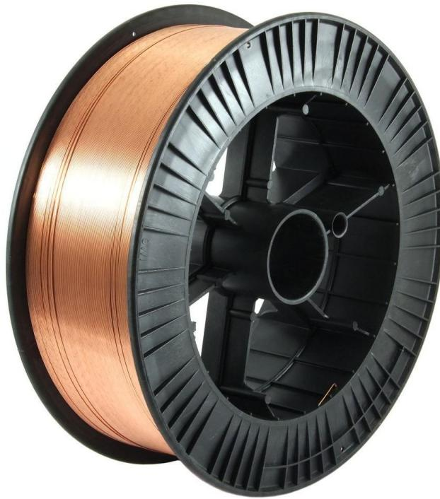
TAURUS MIG SILICON BRONZE is a pure copper filler wire deoxidised with 3% silicon for welding a wide range of copper alloys including overlaying of steels and cast irons. The wire is optimised for laser brazing.
