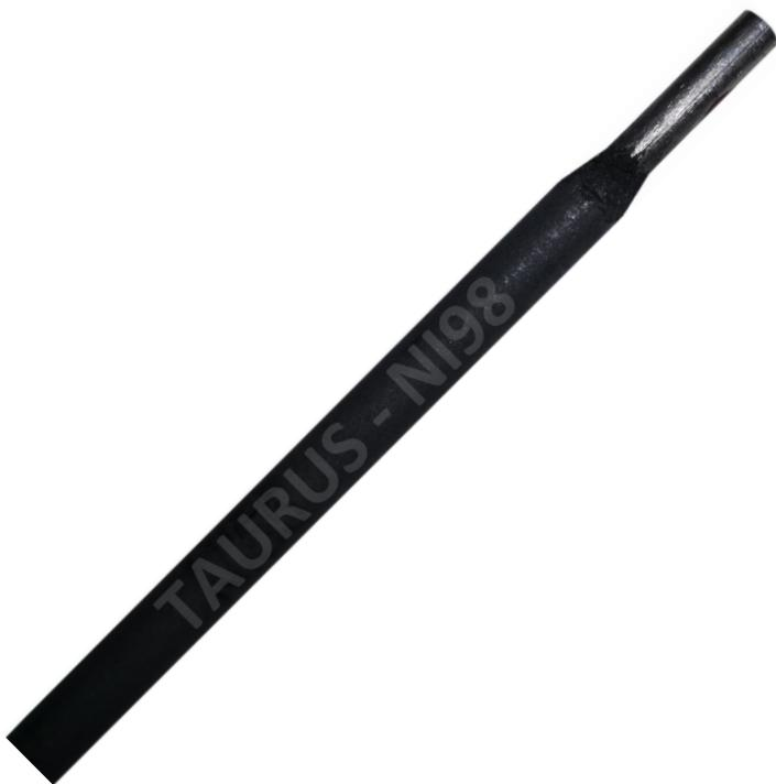
TAURUS PRO Ni 98 is a pure nickel electrode which is universally used for welding all types of cast iron. Specially designed to operate at low currents which minimises heat input and thus facilitates the cold welding of cast iron. Weld-induced stresses can be reduced by hammer peening. Stable arc with clean bead appearance. The weld metal is fully machinable.
