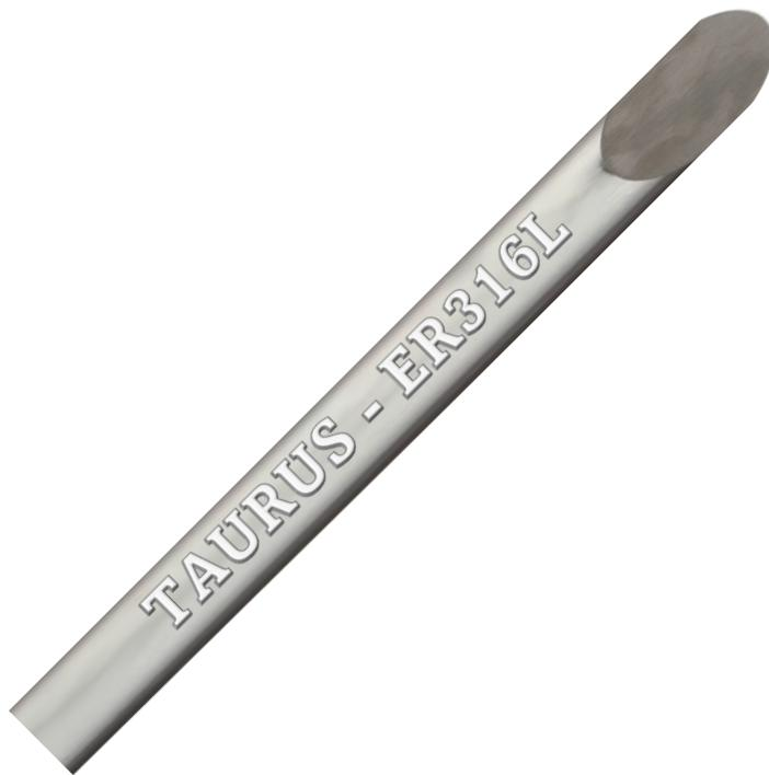
TAURUS TIG 316L rod is used for molybdenum-bearing austenitic stainless steels with 1.5- 3 % molybdenum. Type 316/316L steels are widely used for its good resistance to pitting, many acids and general corrosion.
