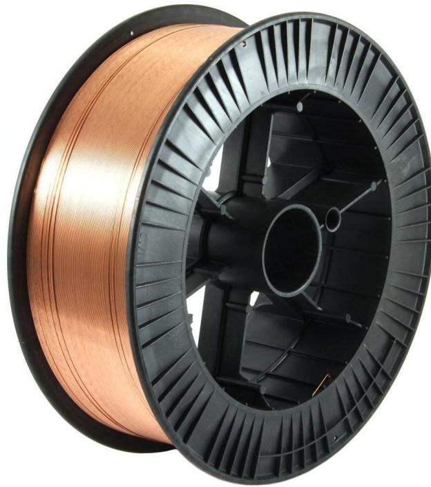
The TAURUS ER70S-6 MIG wire is produced from high quality de-oxidised rod. The products are copper coated for increased shelf life, which facilitates good electrical conductivity with reduced friction during high speed welding. The TAURUS ER70S-6 MIG wire is a premium quality wire which is precision layer-wound to produce positive, uninterrupted feeding in semi-automatic and automated systems.
