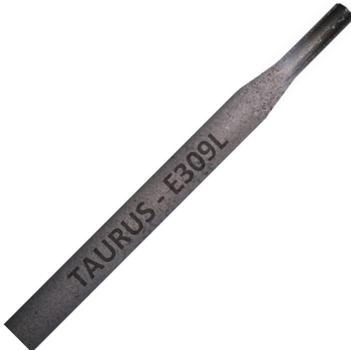
TAURUS PRO 309L is a rutile, extra-low carbon-resistant electrode for welding corrosion resistant and heat resistant CR and CrNi steels. The high level of alloying elements also makes this electrode suitable for welding Cr and CrNi steel to mild steel. Very smooth weld with clean edge, low spatter loss and excellent slag removability.
