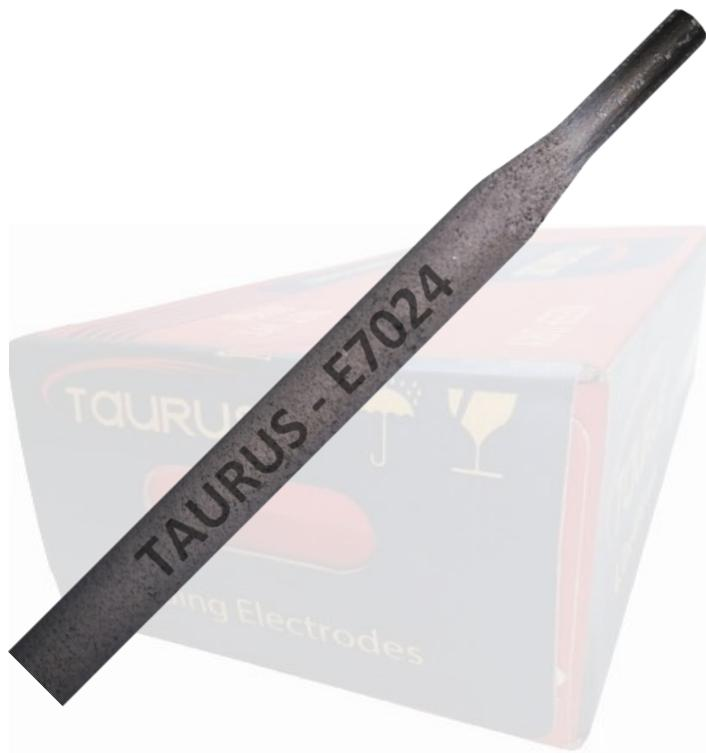
TAURUS PRO 7024 is a rutile, coated-iron, high-recovery electrode which deposits metal of good metallurgical properties quickly and economically. Designed for downhand and fillet welding. TAURUS 7024 has a recovery of approximately 160%. The arc is smooth and consistent with very little spatter. Striking and restriking qualities are excellent.
