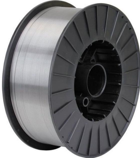
TAURUS E71T-1 is a rutile type CO<sub>2</sub> shielded flux-cored wire for welding carbon-manganese steels. It is recommended for the all positional welding of mild and low-alloy steels with a tensile strength of up to 620 MPa for general purpose fabrication. This wire provides increased toughness at sub zero temperatures.
