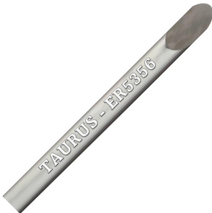
TAURUS TIG 5356 is a 95% aluminium, 5% magnesium rod for general purpose welding when 40 000 psi tensile strength is not required. TAURUS TIG 5356 should be used with a zirconated tungsten electrode with pure argon or an argon-helium mixture for thick sections, at a flow rates of 10 - 15 l/min. For oxy-acetylene gas welding, a neutral flame should be used with aluminium welding flux.
